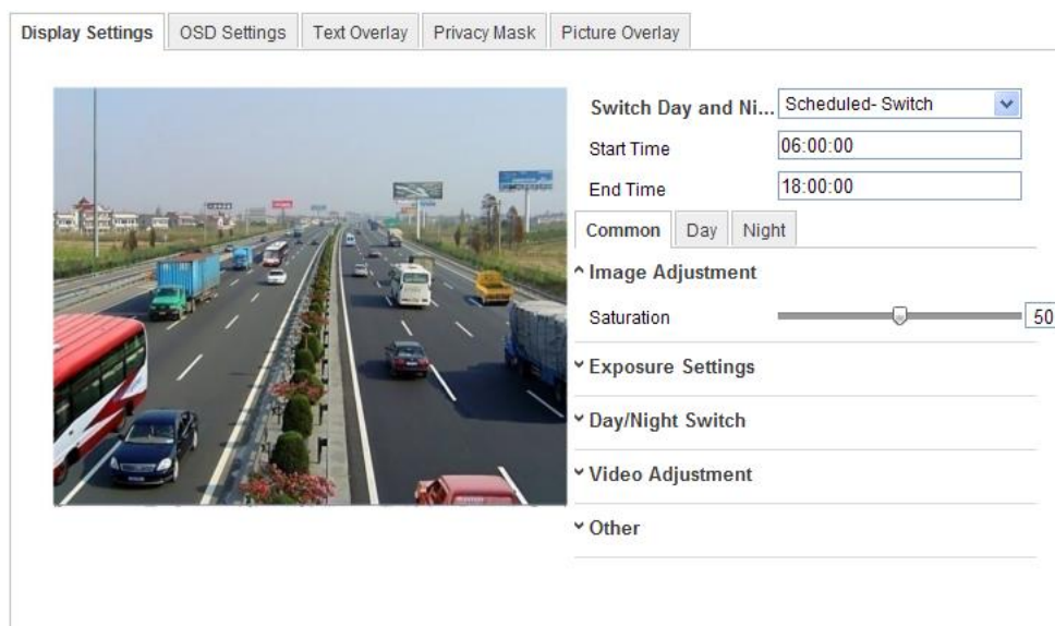
Figure 6-37 Day/Night Scheduled-Switch Configuration Interface
